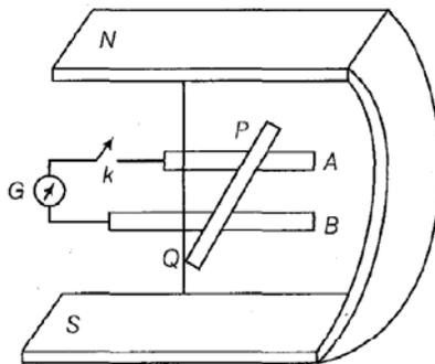
A galvanometer  $G$  connects the rails through a switch  $k$ . Length of the rod  $15\text{ cm}$ ,  $B = 0.50\text{ T}$ , resistance of the closed loop containing the rod  $= 9.0\text{ m}\Omega$ . Assume the field to be uniform.
